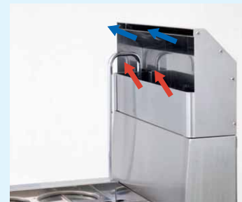
Airflow on the heat insulating layer of a back guard takes heat from the back surface of main body. Exhaust gas can be prevented from spreading.
