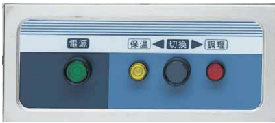
By pressing “Switch” button, the lamp shows Cook or Keep Warm.
