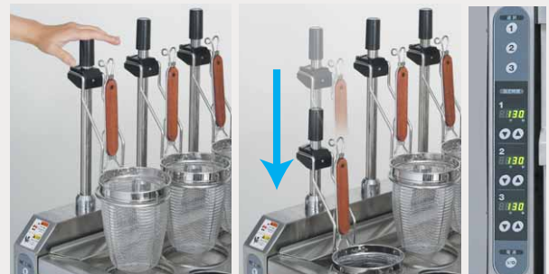
Lift down when you push the Lift Cap.
